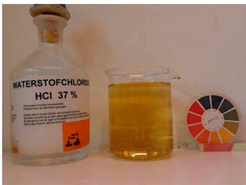
Figure 5. \text{SrSO}_3 precipitation disappears after addition of HCl to the wine solution.
