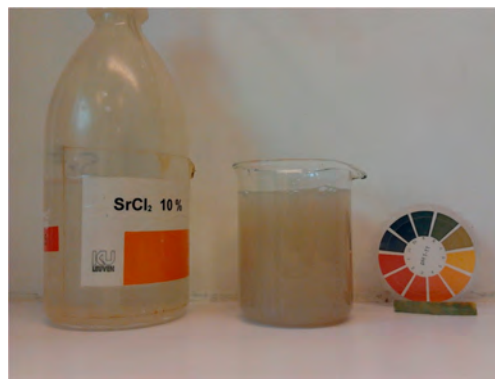
Figure 4. After addition of strontium chloride to a base wine solution, a \text{SrSO}_3 precipitation is formed.
