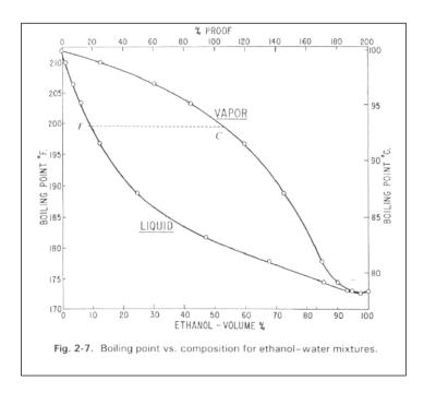
The above diagram illustrates the boiling point versus composition relationship for the water-ethanol system.
